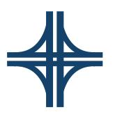
**Split-diamond interchange:** A split-diamond interchange is a diamond interchange in which the two halves of the diamond are separated along the freeway by two lengths of frontage road. There might be additional intersections between the freeway on ramps and off ramps
