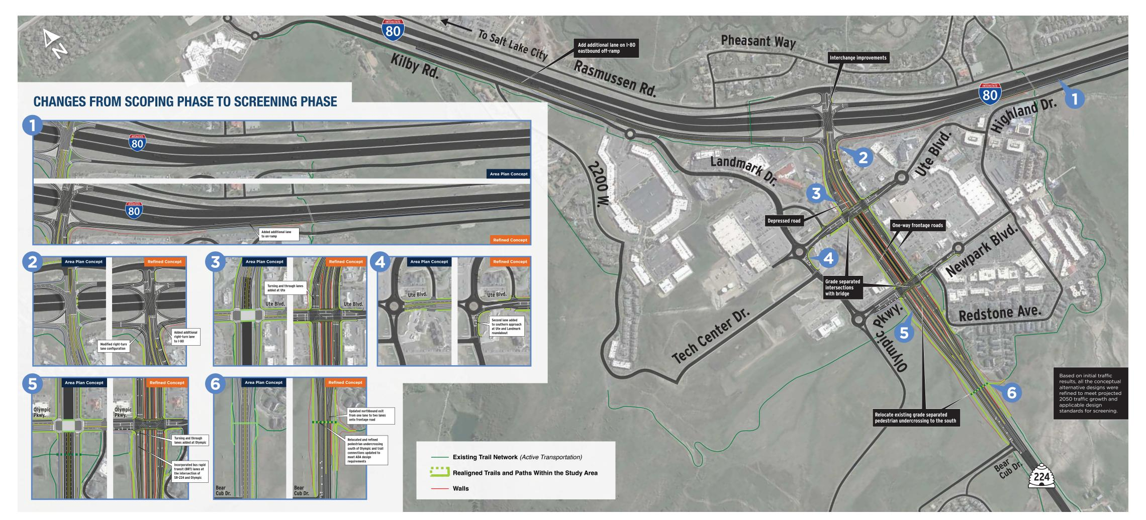
ALTERNATIVE B: GRADE-SEPARATED INTERSECTIONS WITH ONE-WAY FRONTAGE ROADS TO THE I-80 INTERCHANGE
