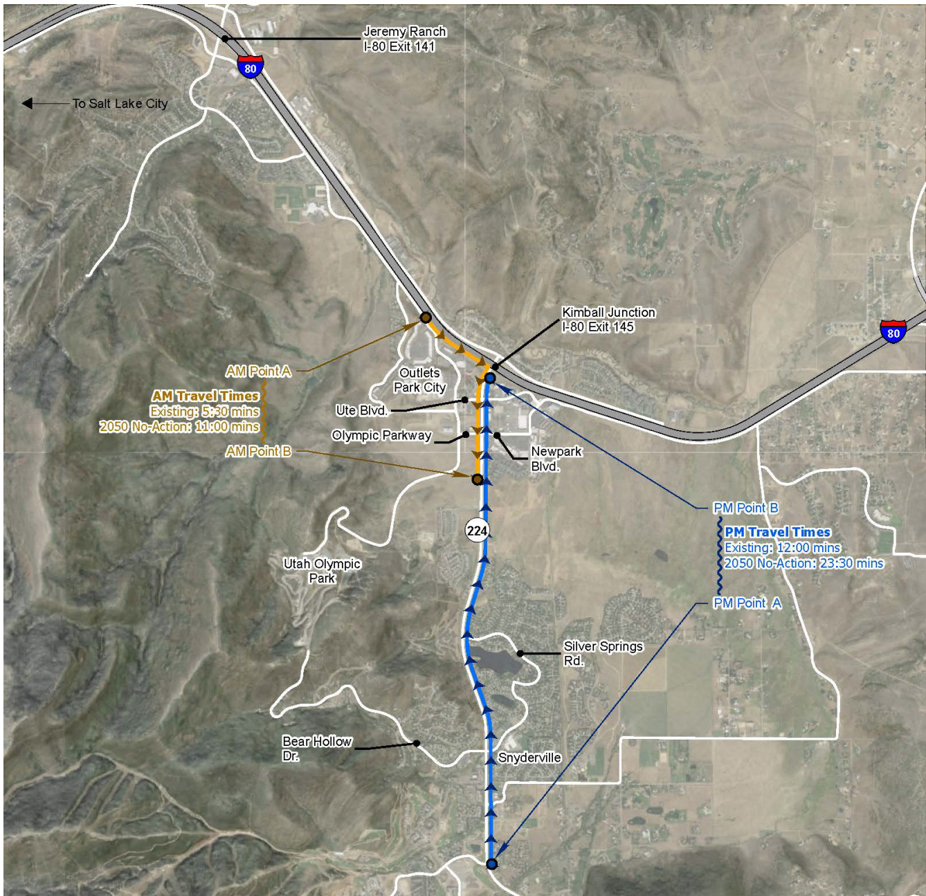
Figure 1.4-4. Travel Times for the Existing (2022) and No-action (2050) Conditions during the AM and PM Peak Hours
