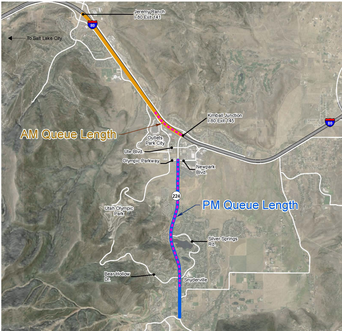
Figure 1.4-5. Vehicle Queue Lengths for the Existing (2022) and No-action (2050) Conditions during the AM and PM Peak Hours
