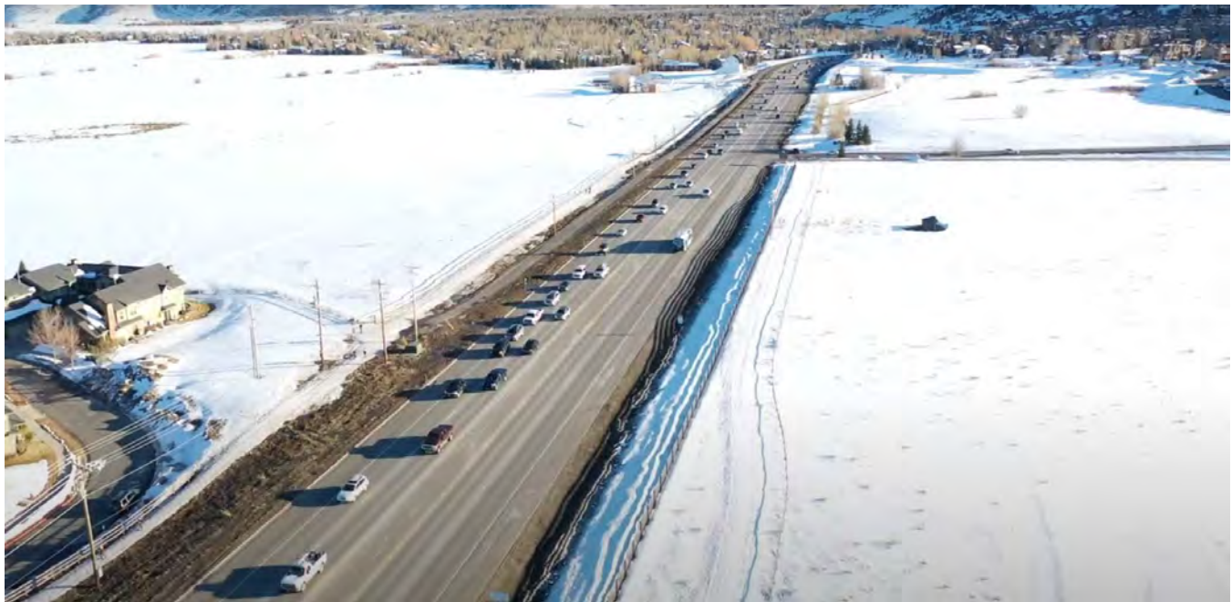
Figure 3: Northbound SR-224 Weekday PM Peak Hour Queues, Looking South from 850 Feet North of Bear Cub Road
